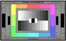
and the blacks are the same. A good way to see this is to have the cameras going through a switcher and have the switcher set to a vertical wipe where the horizontal line moves up and down to create the transition. While focused on the gray chart, now is a good time to white balance the cameras.
